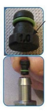
The size of each dosing restrictor nozzle is marked on the lip
